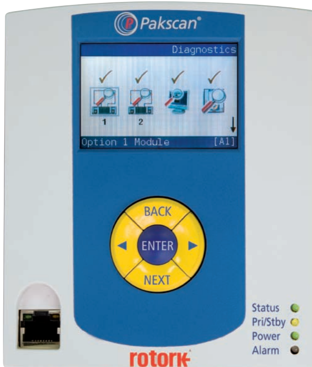
CPU module with colour graphical HMI
