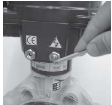
Setting clockwise to close stop bolt
