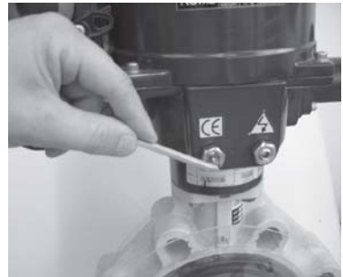
Setting anti-clock to close stop bolt
