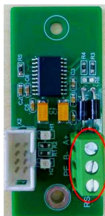
Figure 10 Terminals Supported by the Actuators (Easytrac)
