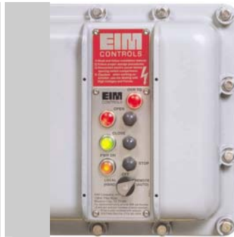
LOCAL/OFF/REMOTE 就地/停止/远程选择开关 OPEN/CLOSE/STOP 打开/关闭/停止按钮
