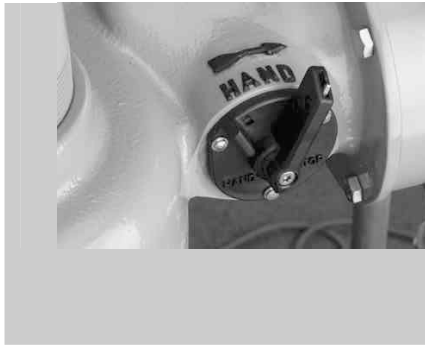
HAND/MOTOR CLUTCH LEVER 手动/电动离合器切换手柄
