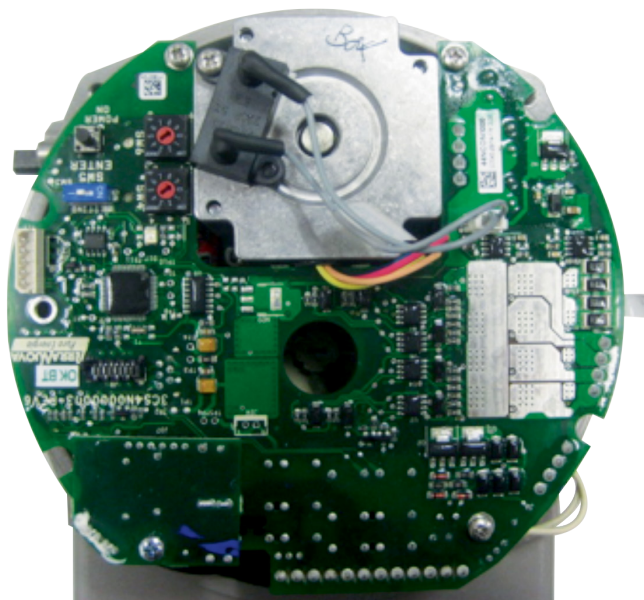
Figure 37. Example of SCE300 New Version (Heat Sink Not Present)
