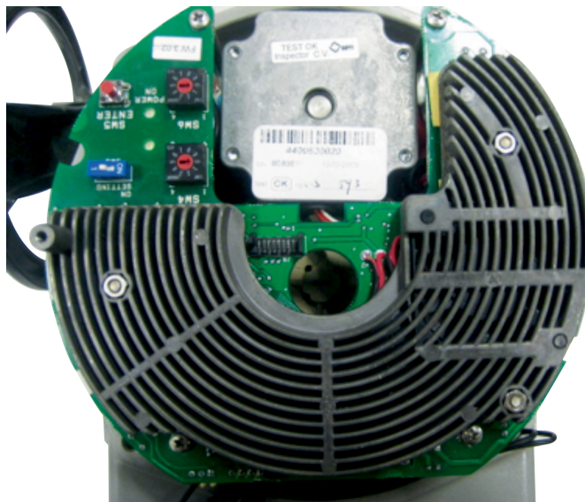
Figure 36. Example of SCE300 Old Version (Heat Sink Present)
