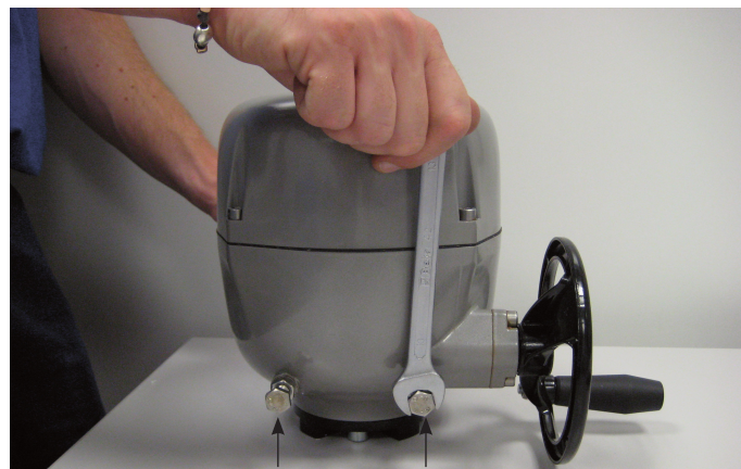
Figure 8. Setting of the Mechanical Stop
