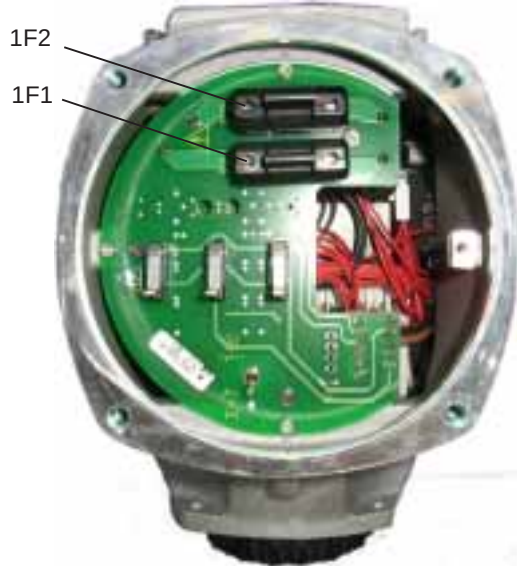
Figure U1: Fuses on signal and control board
